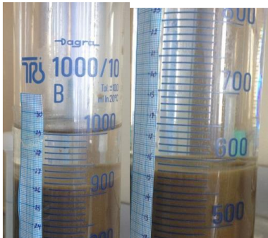
Figure 2 – Height of the clarified layer 4 hours (1) and 24 hours (2) after sedimentation of industrial wastewater
